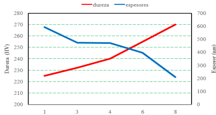
Figure 8. Hardness vs. thickness behavior.
